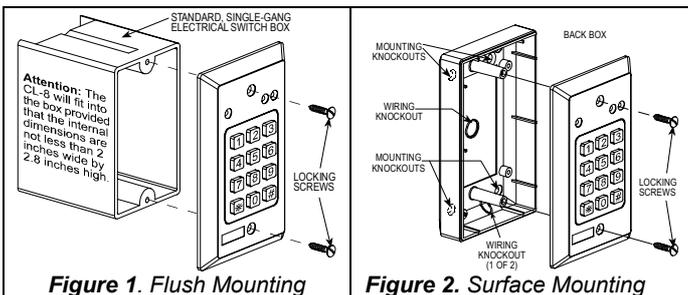
Figure 1. Flush Mounting
